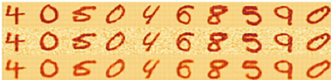
Fig. 14.15 Visualization of 10 randomly selected digits (test data) used for predicting the output of an autoencoder. The original digits are shown at the top row and the noisy digits used for training in the middle row, and the output of the denoising autoencoder (as produced by Listing 14.7) is shown in the bottom row
