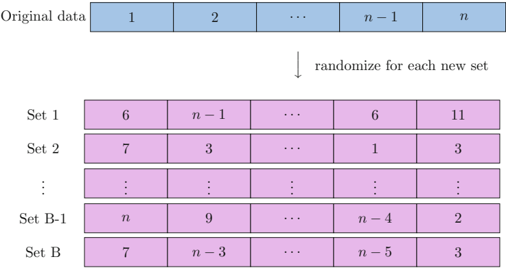
Fig. 4.3 Visualization of bootstrap. The method generates B new data sets with B \in \mathbb{N} that can be larger than n . Each of these B data sets is generated by drawing n samples with replacement. This means that it is possible for data points to appear many times in a new data set (see the value “3” in Set 2)
