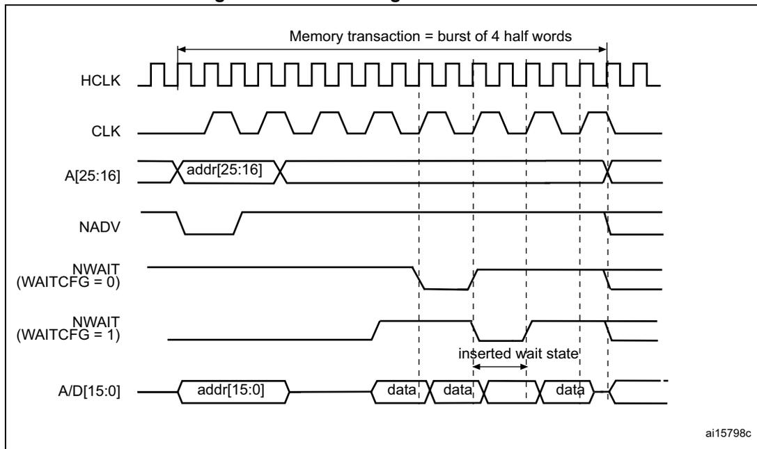
Figure 472. Synchronous multiplexed read mode waveforms - NOR, PSRAM (CRAM)
