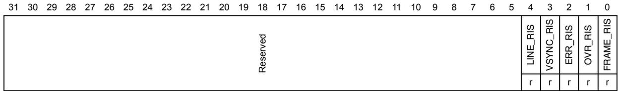
DCMI\_RIS gives the raw interrupt status and is accessible in read only. When read, this register returns the status of the corresponding interrupt before masking with the DCMI\_IER register value.
