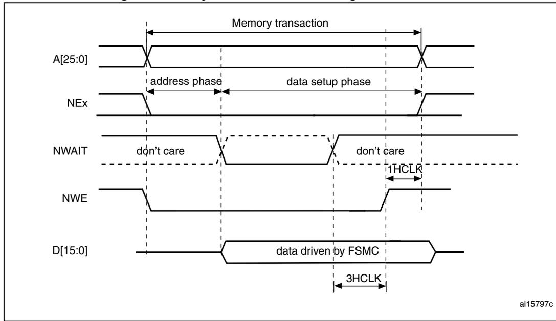
1. NWAIT polarity depends on WAITPOL bit setting in FSMC\_BCRx register.
