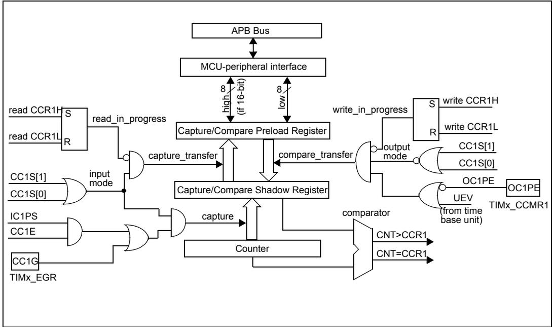
Figure 161. Output stage of capture/compare channel (channel 1)
