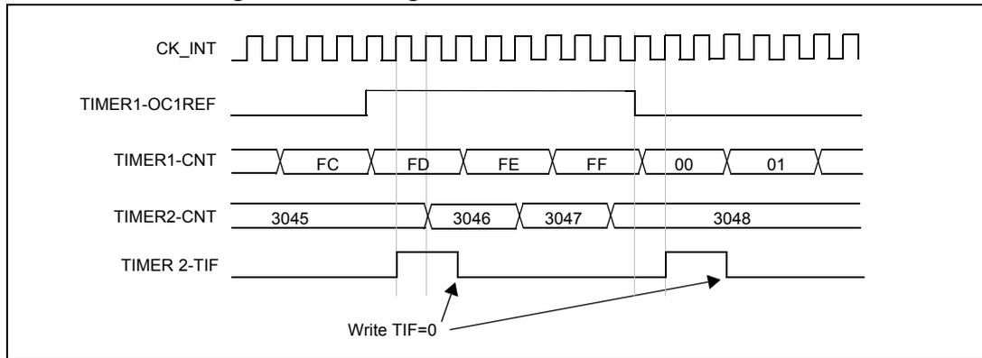
In the example in [Figure 241](#), the Timer 2 counter and prescaler are not initialized before being started. So they start counting from their current value. It is possible to start from a given value by resetting both timers before starting Timer 1. You can then write any value you want in the timer counters. The timers can easily be reset by software using the UG bit in the TIMx\_EGR registers.
