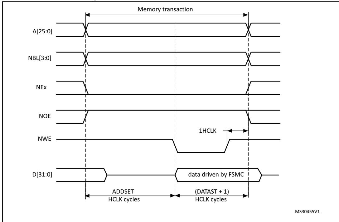
The differences compared with mode1 are the toggling of NOE and the independent read and write timings.
