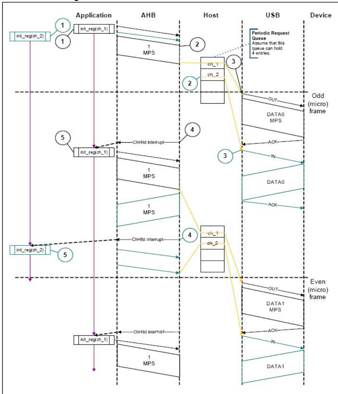
Figure 419. Bulk/control IN transactions - Slave mode
