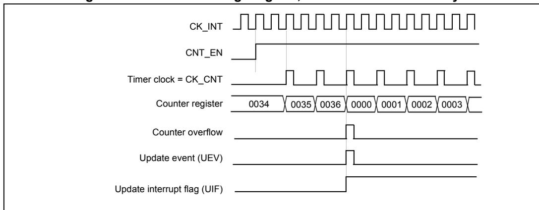
**Figure 139. Counter timing diagram, internal clock divided by 4**
