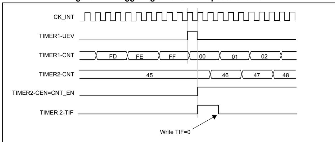
As in the previous example, you can initialize both counters before starting counting. [Figure 178](#) shows the behavior with the same configuration as in [Figure 241](#) but in trigger mode instead of gated mode (SMS=110 in the TIM2\_SMCR register).
