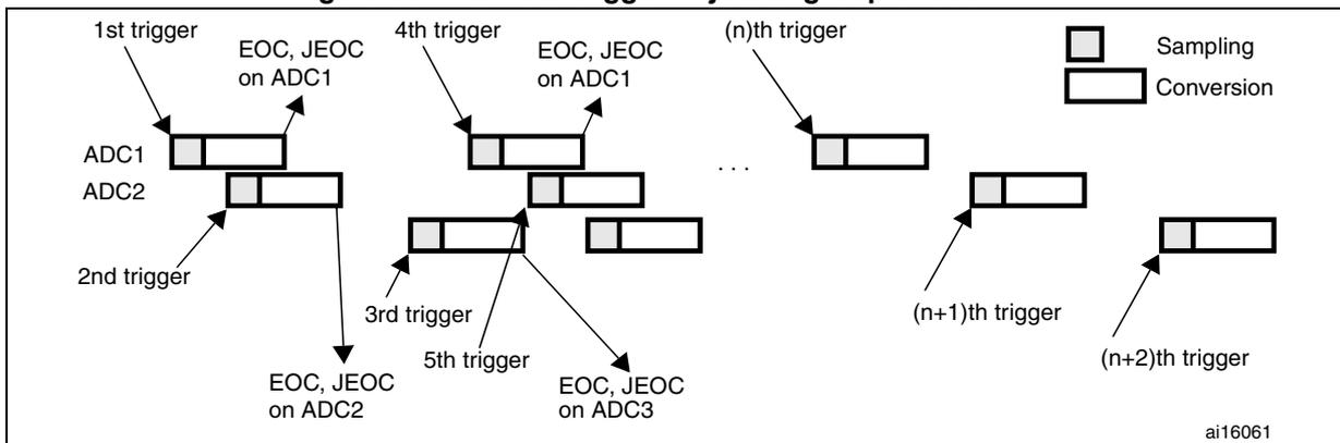
**13.9.5 Combined regular/injected simultaneous mode**
