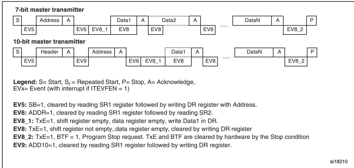
1. The EV5, EV6, EV9, EV8\_1 and EV8\_2 events stretch SCL low until the end of the corresponding software sequence.
