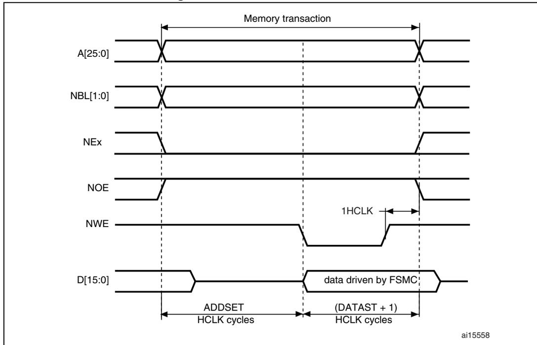
The one HCLK cycle at the end of the write transaction helps guarantee the address and data hold time after the NWE rising edge. Due to the presence of this one HCLK cycle, the DATAST value must be greater than zero (DATAST > 0).
