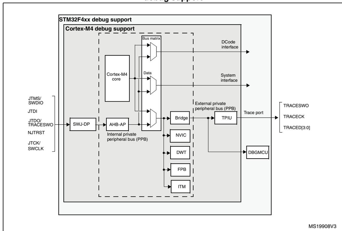
*Note:* The debug features embedded in the Cortex<sup>®</sup>-M4 with FPU core are a subset of the ARM<sup>®</sup> CoreSight Design Kit.
