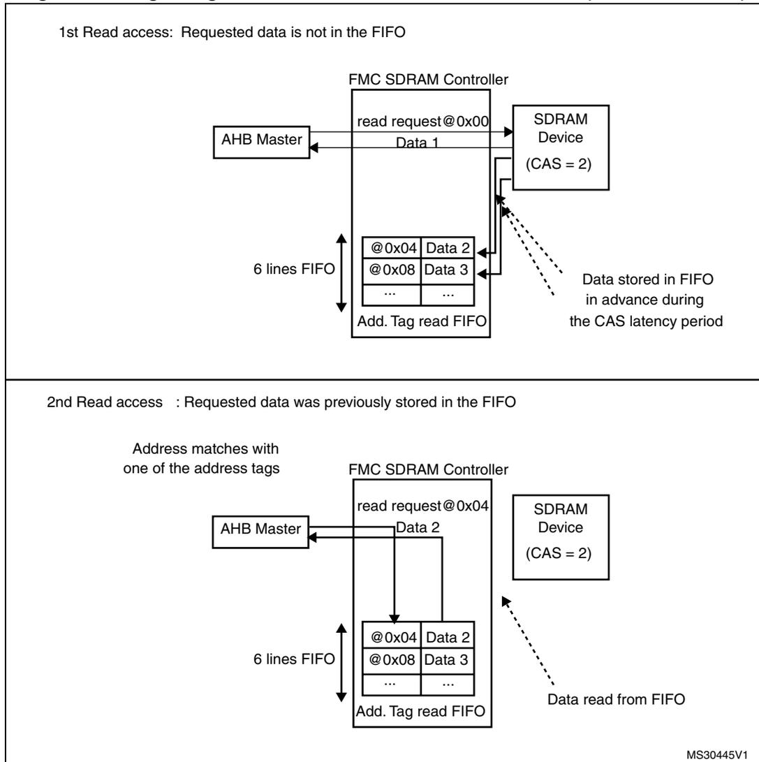
During a write access or a Precharge command, the read FIFO is flushed and ready to be filled with new data.
