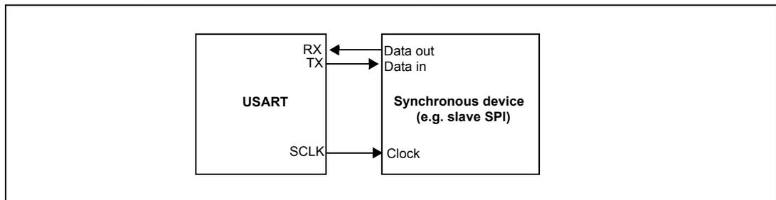
Figure 308. USART data clock timing diagram (M=0)
