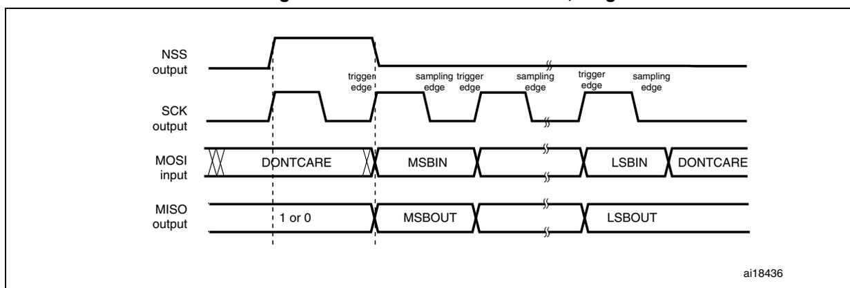
**Figure 252. TI mode - master mode, continuous transfer**
