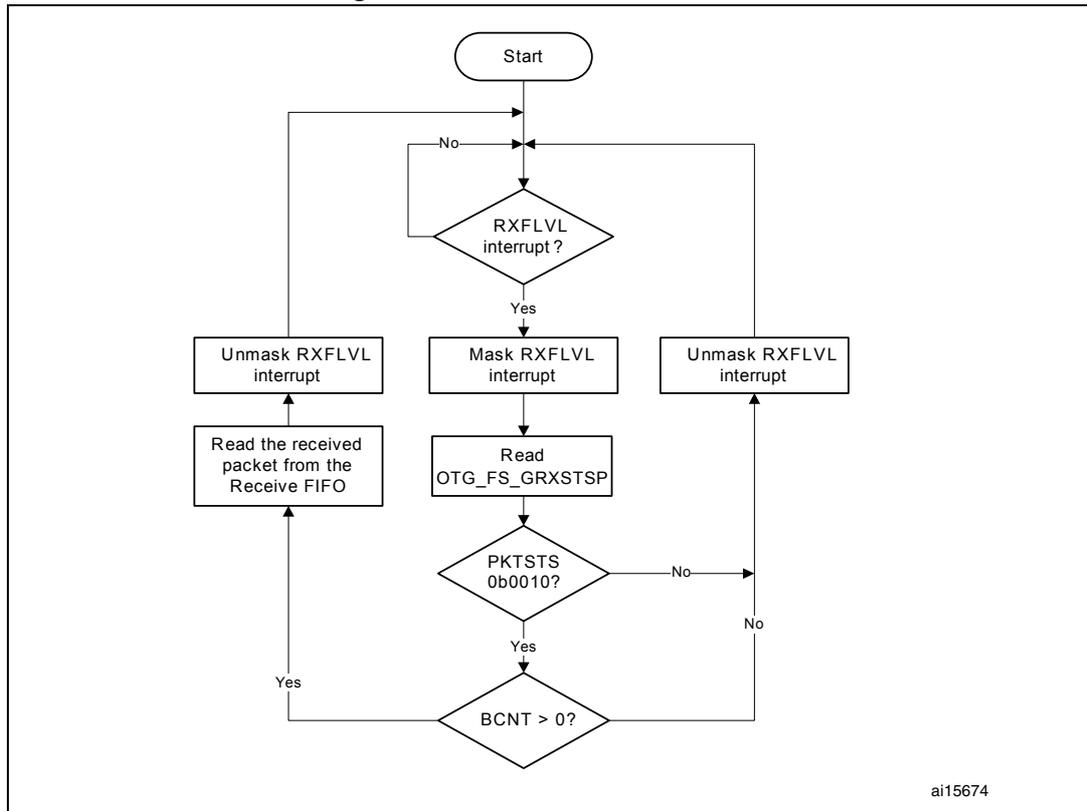
• **Bulk and control OUT/SETUP transactions**
