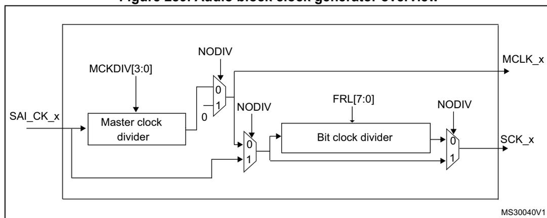
**Note:** *If NoDiv is set to 1, the MCLK\_x signal will be set at 0 level if this pin is configured as the SAI pin in GPIO peripherals.*
