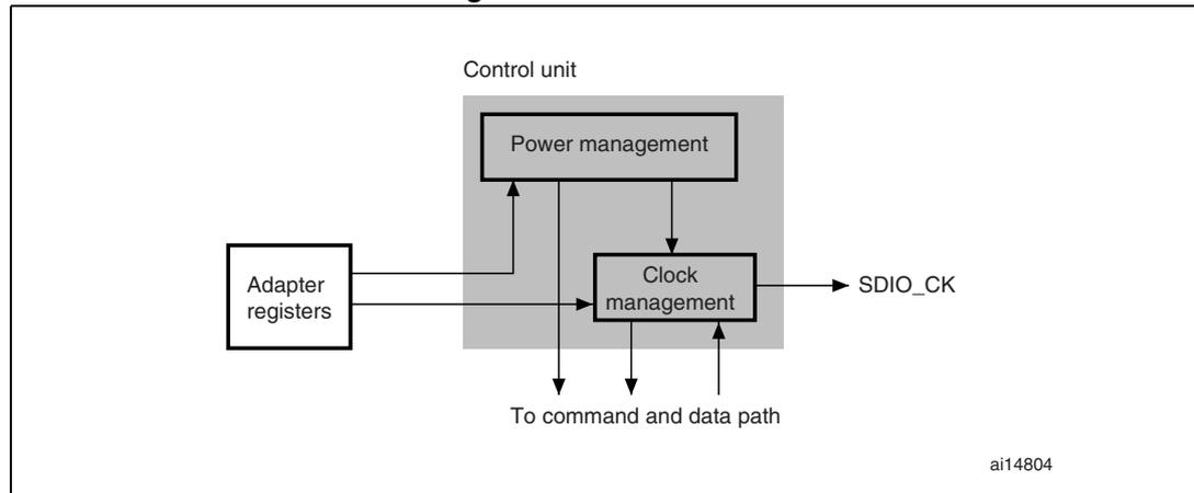
The control unit is illustrated in [Figure 328](#). It consists of a power management subunit and a clock management subunit.
