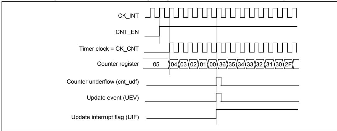
**Figure 144. Counter timing diagram, internal clock divided by 2**
