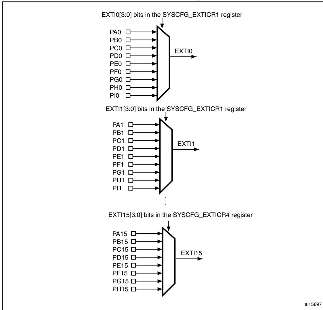
**Figure 43. External interrupt/event GPIO mapping (STM32F42xxx and STM32F43xxx)**
