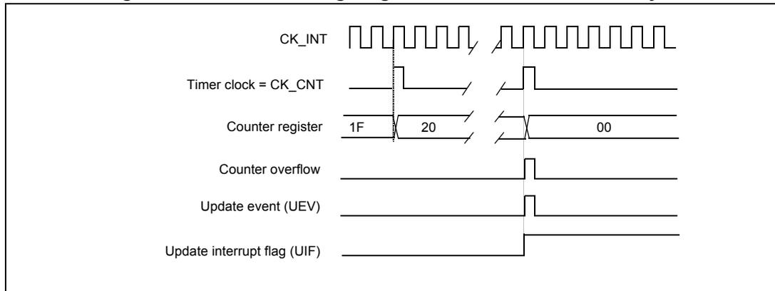
Figure 141. Counter timing diagram, Update event when ARPE=0 (TIMx\_ARR not preloaded)
