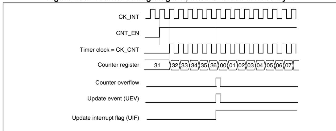
**Figure 207. Counter timing diagram, internal clock divided by 2**
