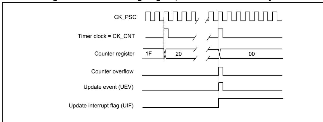
**Figure 93. Counter timing diagram, update event when ARPE=0 (TIMx\_ARR not preloaded)**
