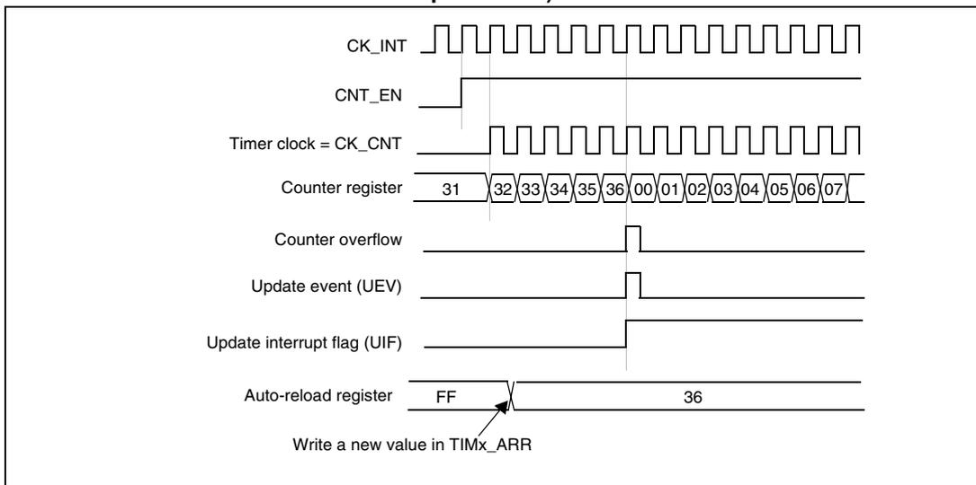
**Figure 211. Counter timing diagram, update event when ARPE=1 (TIMx\_ARR preloaded)**
