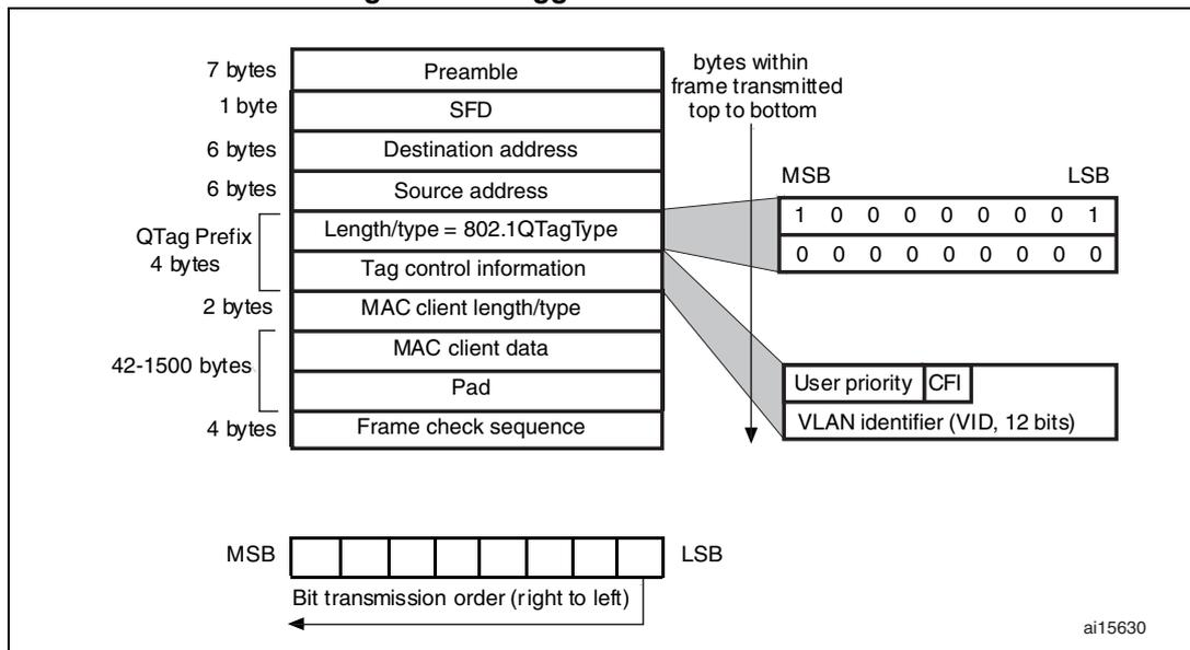
Each byte of the MAC frame, except the FCS field, is transmitted low-order bit first.
