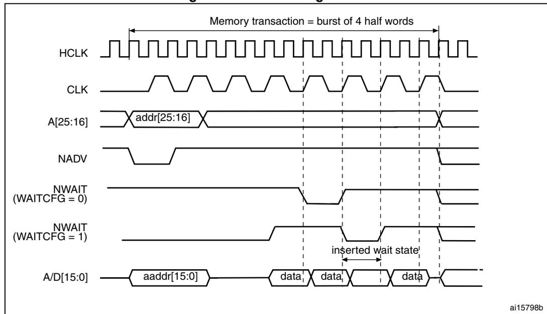
Figure 450. Synchronous multiplexed read mode - NOR, PSRAM (CRAM)
