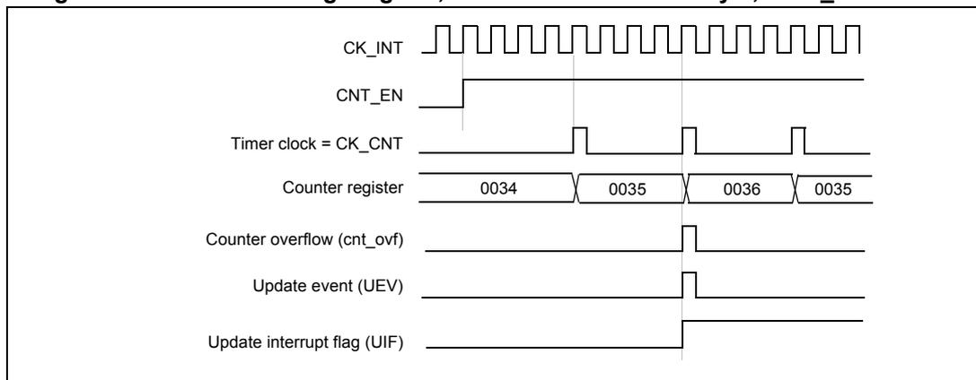
1. Center-aligned mode 2 or 3 is used with an UIF on overflow.
