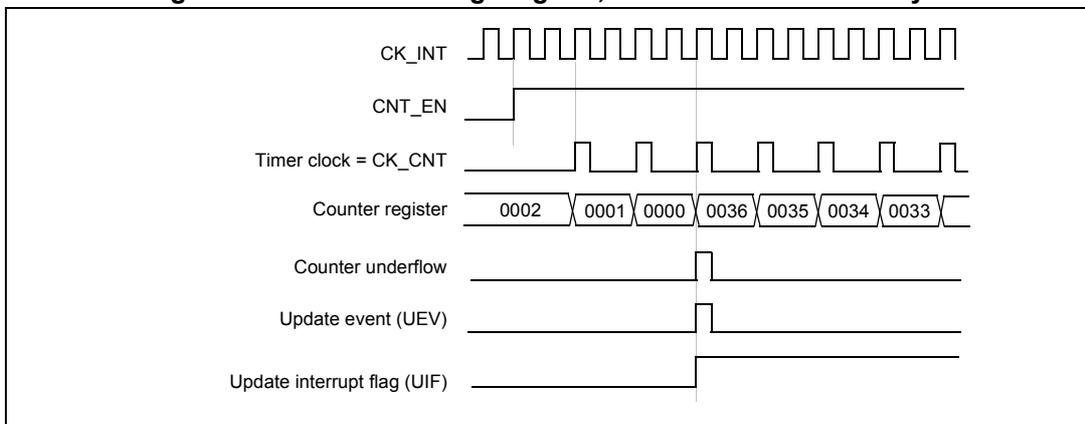
**Figure 145. Counter timing diagram, internal clock divided by 4**
