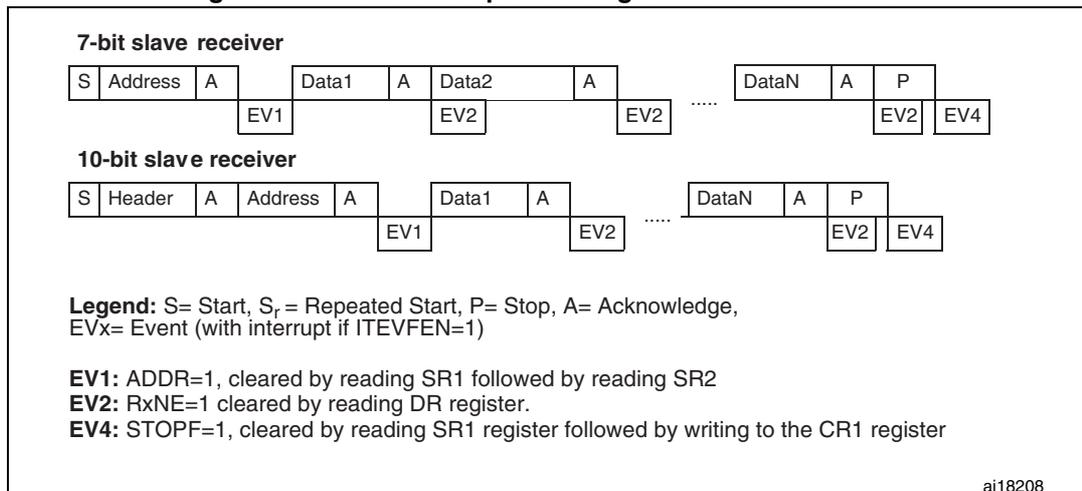
1. The EV1 event stretches SCL low until the end of the corresponding software sequence.
