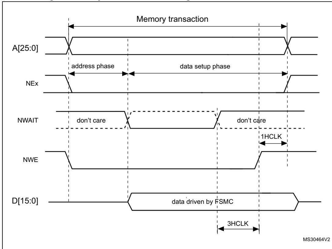
1. NWAIT polarity depends on WAITPOL bit setting in FMC\_BCRx register.
