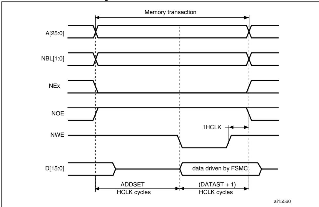
The differences compared with mode1 are the toggling of NOE and the independent read and write timings.
