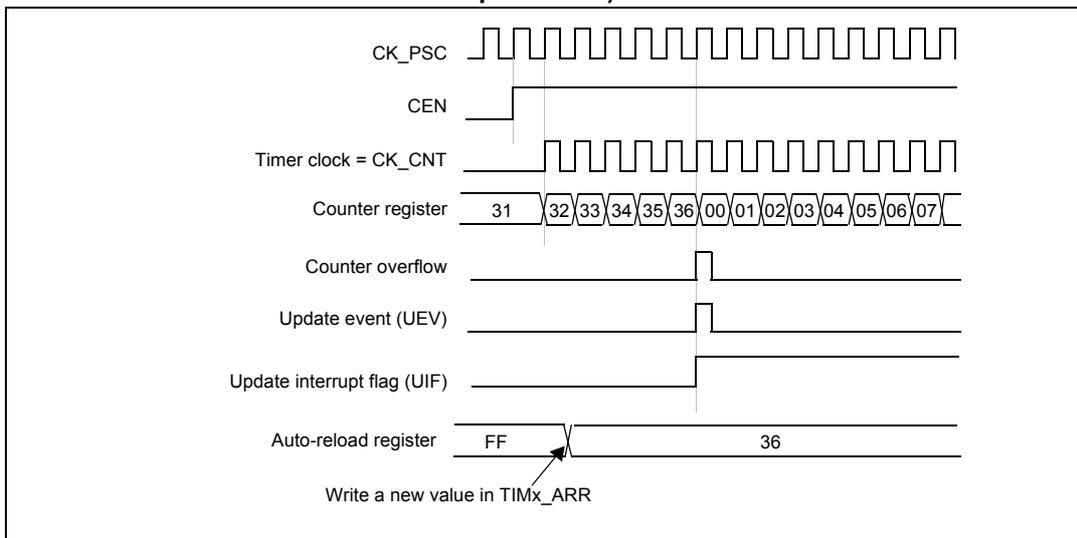
**Figure 189. Counter timing diagram, update event when ARPE=1 (TIMx\_ARR preloaded)**
