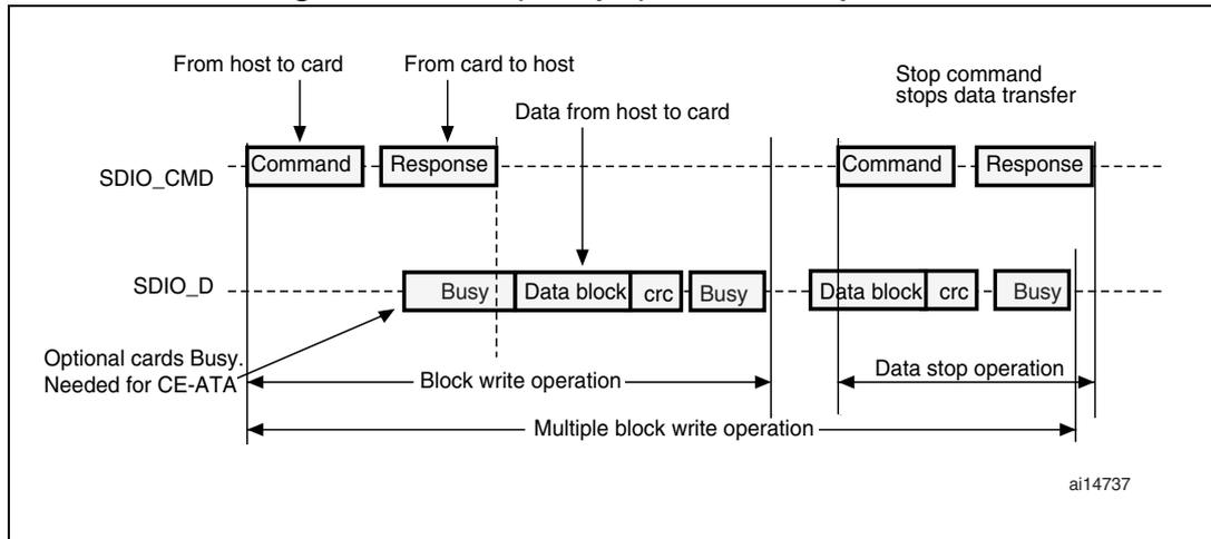
Note: The SDIO will not send any data as long as the Busy signal is asserted (SDIO\_D0 pulled low).
