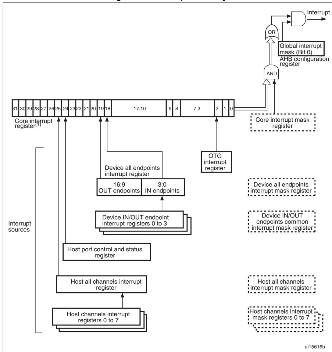
1. The core interrupt register bits are shown in *OTG\_FS core interrupt register (OTG\_FS\_GINTSTS)* on page 1262.
