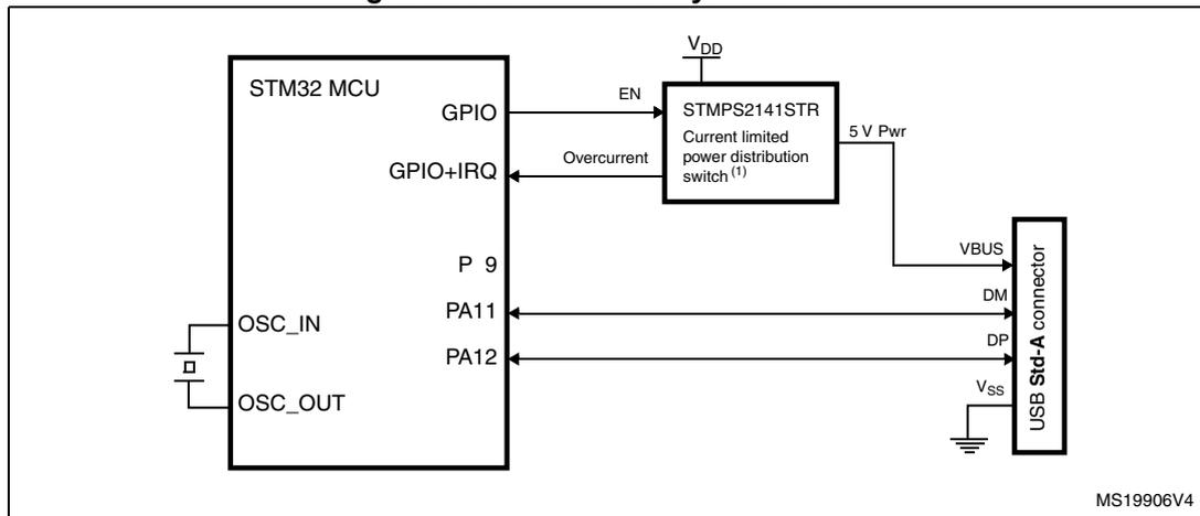
1. STMPS2141STR needed only if the application has to support a  $V_{BUS}$  powered device. A basic power switch can be used if 5 V are available on the application board.
