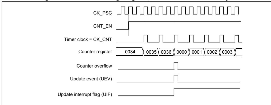
**Figure 91. Counter timing diagram, internal clock divided by 4**
