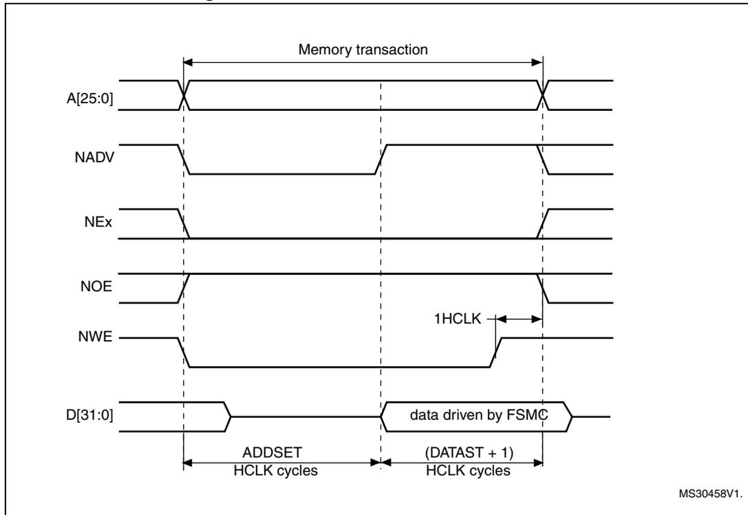
The differences with mode1 are the toggling of NWE and the independent read and write timings when extended mode is set (Mode B).
