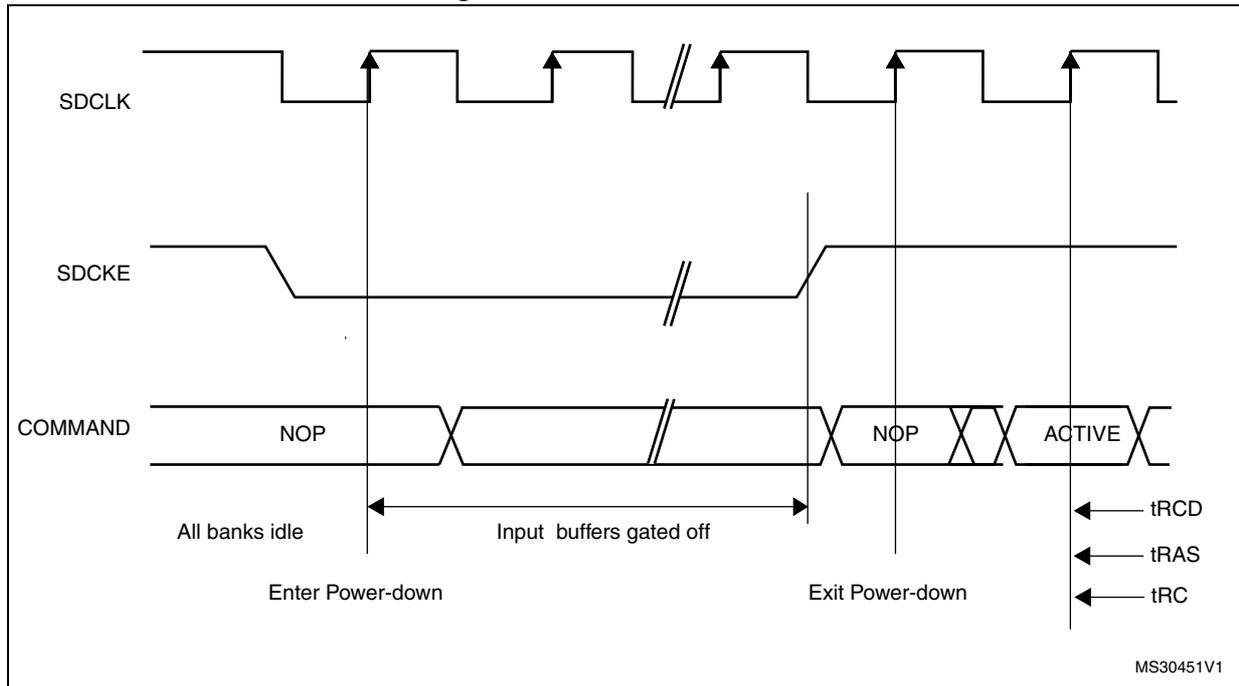
If the Write data FIFO is not empty, all data are sent to the memory before activating the Power-down mode.
