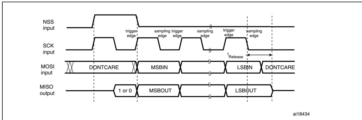
**Figure 250. TI mode - Slave mode, continuous transfer**
