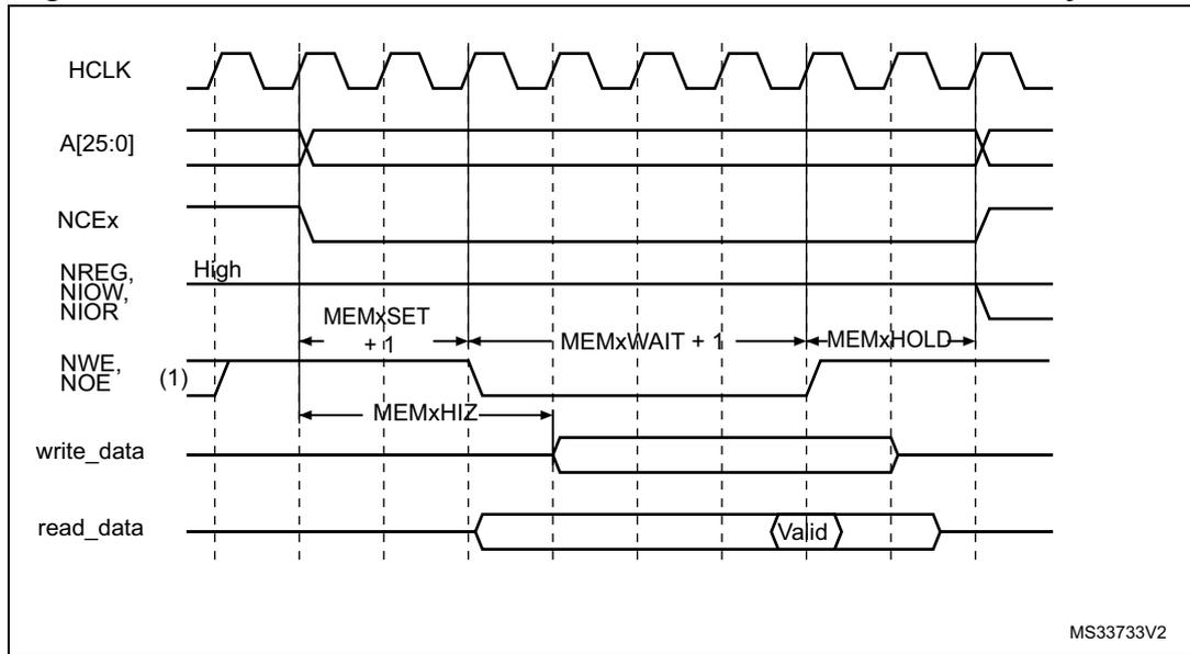
1. NOE remains high (inactive) during write accesses. NWE remains high (inactive) during read accesses.
