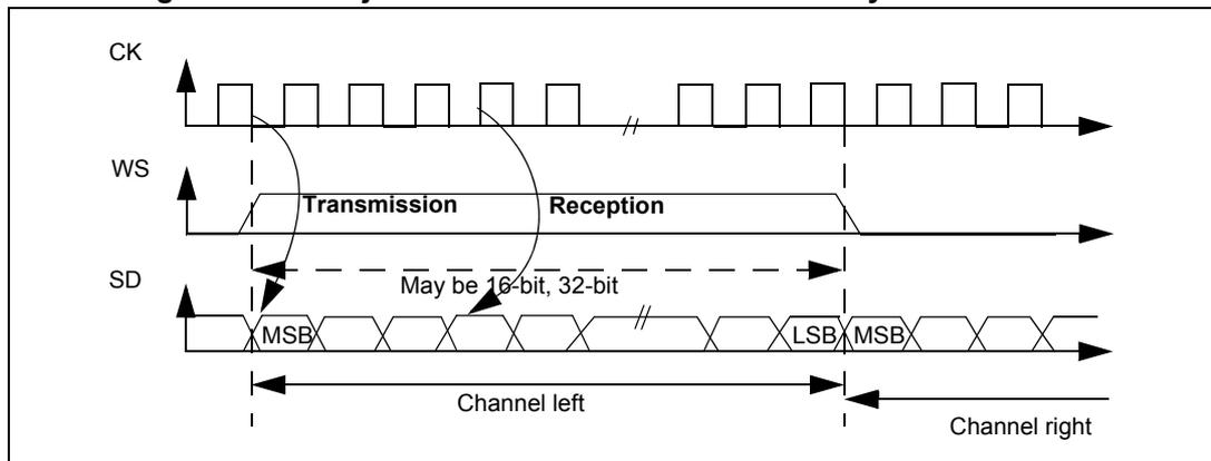
Figure 274. LSB Justified 24-bit frame length with CPOL = 0
