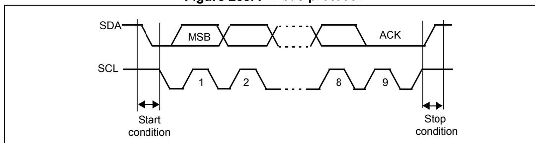
Acknowledge may be enabled or disabled by software. The I<sup>2</sup>C interface addresses (dual addressing 7-bit/ 10-bit and/or general call address) can be selected by software.
