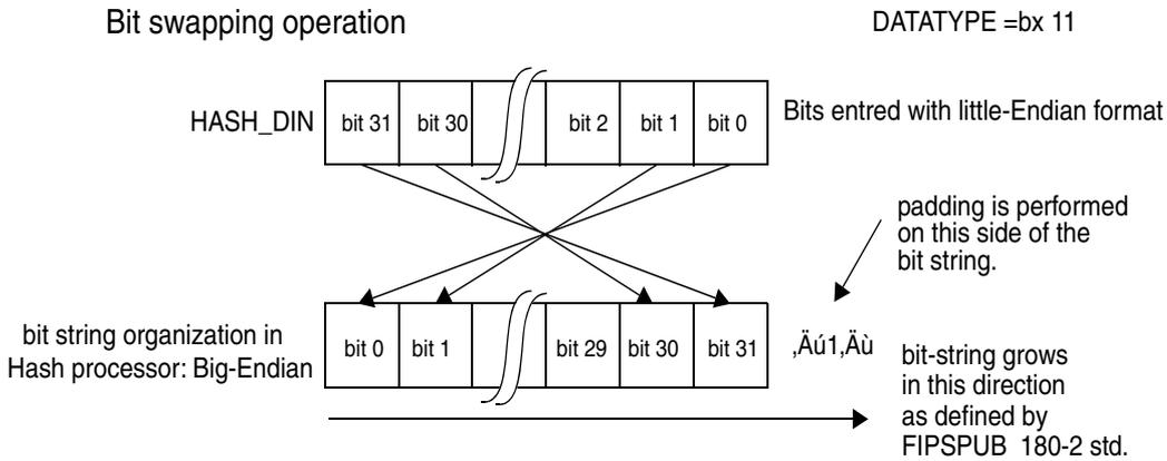
B-In case of byte data hash, all bytes should be swapped as below
