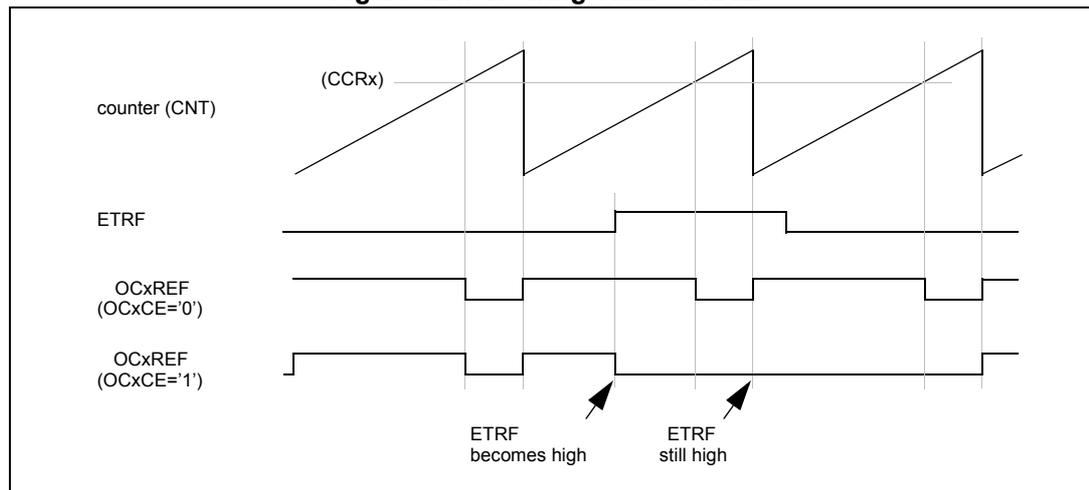
Note: In case of a PWM with a 100% duty cycle (if CCRx>ARR), then OCxREF is enabled again at the next counter overflow.
