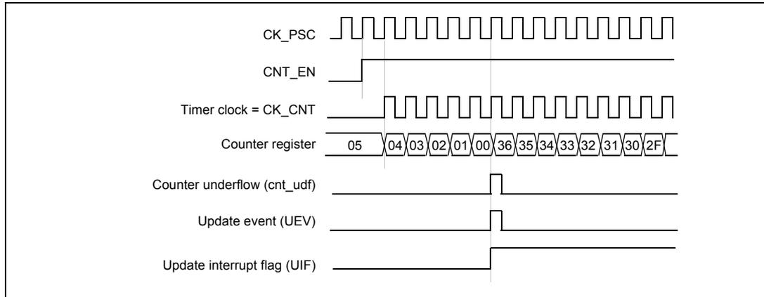
**Figure 96. Counter timing diagram, internal clock divided by 2**
