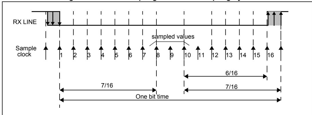
**Figure 302. Data sampling when oversampling by 8**
