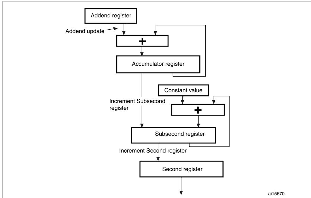
The system time update logic requires a 50 MHz clock frequency to achieve 20 ns accuracy. The frequency division is the ratio of the reference clock frequency to the required clock frequency. Hence, if the reference clock (HCLK) is, let us say, 66 MHz, the ratio is calculated as 66 MHz/50 MHz = 1.32. Hence, the default addend value to be set in the register is  $2^{32}/1.32$ , which is equal to 0xC1F0 7C1F.
