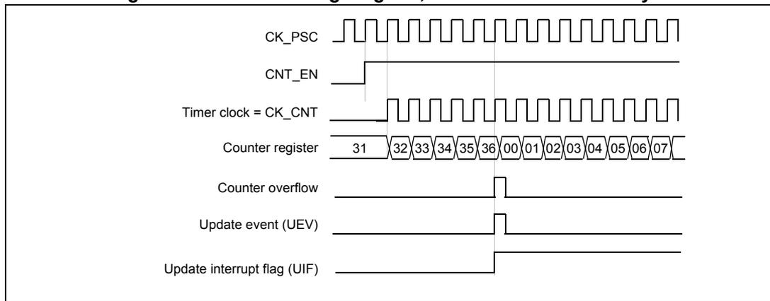
**Figure 90. Counter timing diagram, internal clock divided by 2**
