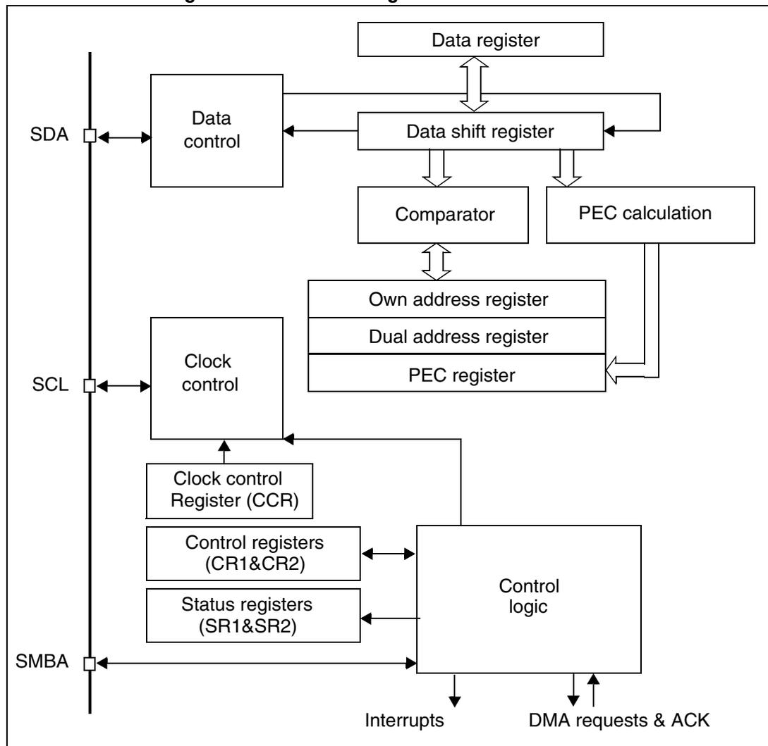
Figure 240. I<sup>2</sup>C block diagram for STM32F42x/43x
