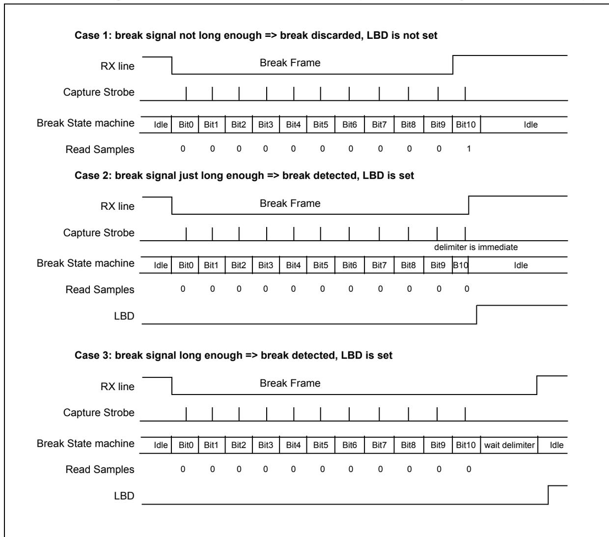
Figure 306. Break detection in LIN mode vs. Framing error detection
