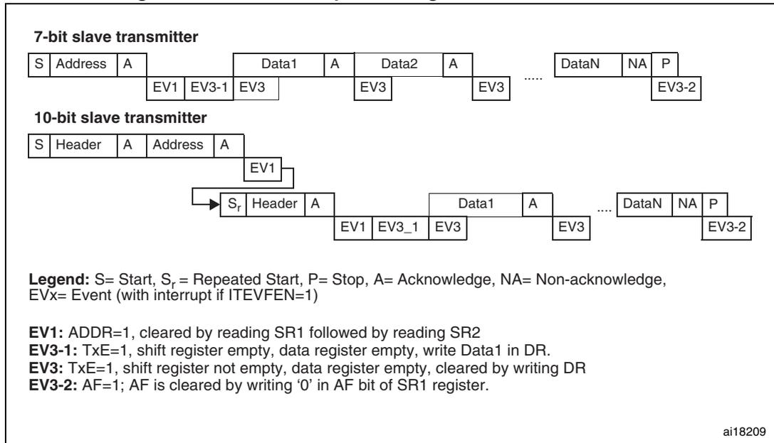
1. The EV1 and EV3\_1 events stretch SCL low until the end of the corresponding software sequence.
