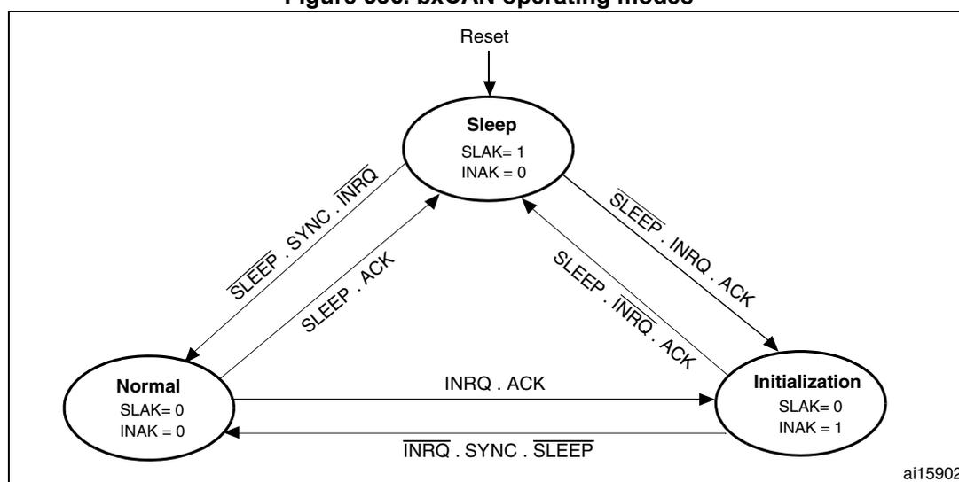
1. ACK = The wait state during which hardware confirms a request by setting the INAK or SLAK bits in the CAN\_MSR register
