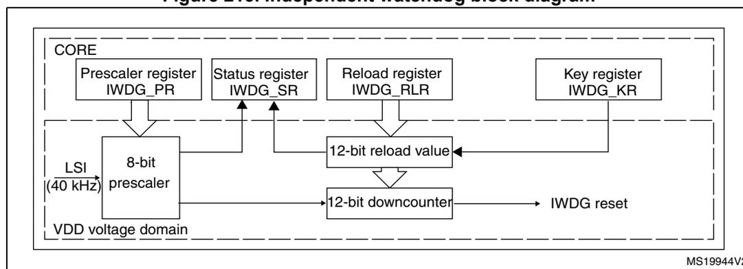
Note: The watchdog function is implemented in the  $V_{DD}$  voltage domain that is still functional in Stop and Standby modes.
