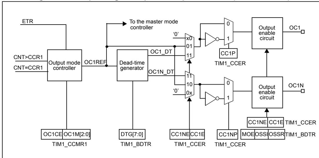
Figure 115. Output stage of capture/compare channel (channel 4)
