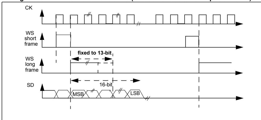
*Note:* For both modes (master and slave) and for both synchronizations (short and long), the number of bits between two consecutive pieces of data (and so two synchronization signals) needs to be specified (DATLEN and CHLEN bits in the SPI\_I2SCFGR register) even in slave mode.
