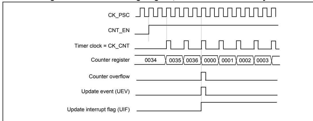
Figure 186. Counter timing diagram, internal clock divided by 4
