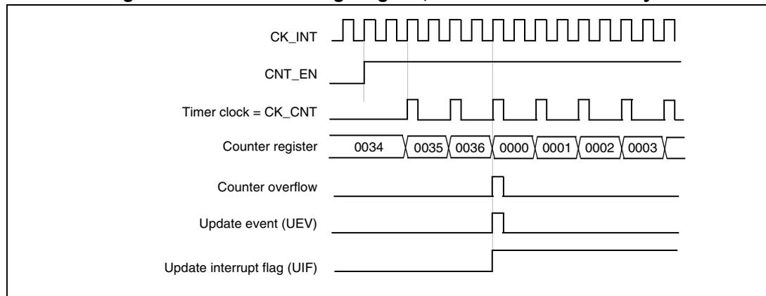
**Figure 208. Counter timing diagram, internal clock divided by 4**
