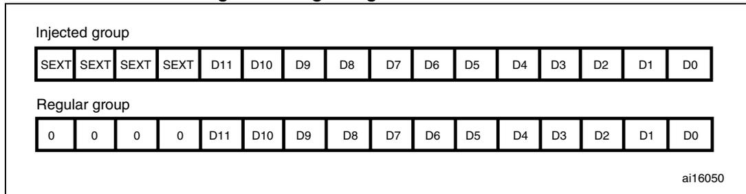
**Figure 49. Left alignment of 12-bit data**
