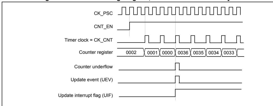
**Figure 97. Counter timing diagram, internal clock divided by 4**
