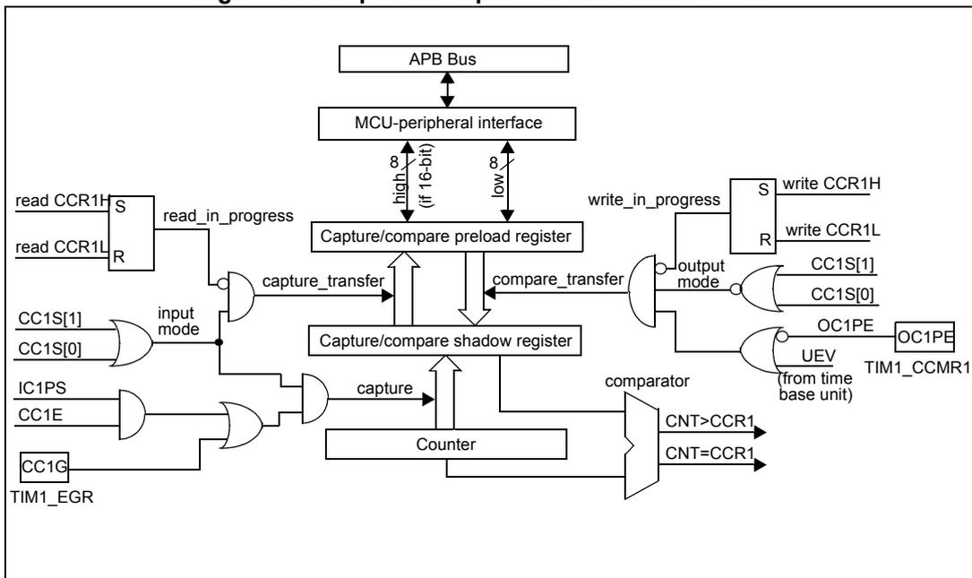
Figure 114. Output stage of capture/compare channel (channel 1 to 3)
