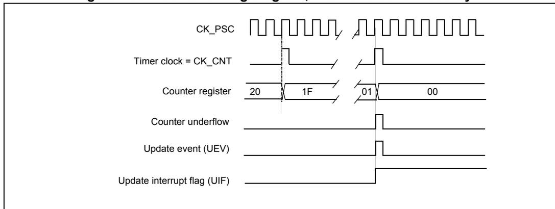
**Figure 104. Counter timing diagram, update event with ARPE=1 (counter underflow)**
