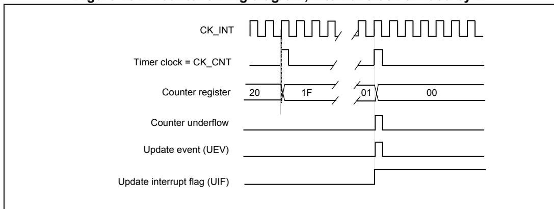
**Figure 152. Counter timing diagram, Update event with ARPE=1 (counter underflow)**
