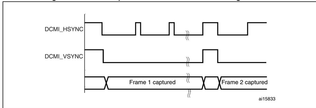
1. Here, the active state of DCMI\_HSYNC and DCMI\_VSYNC is 1.
