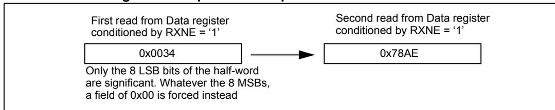
**Figure 277. LSB justified 16-bit extended to 32-bit packet frame with CPOL = 0**
