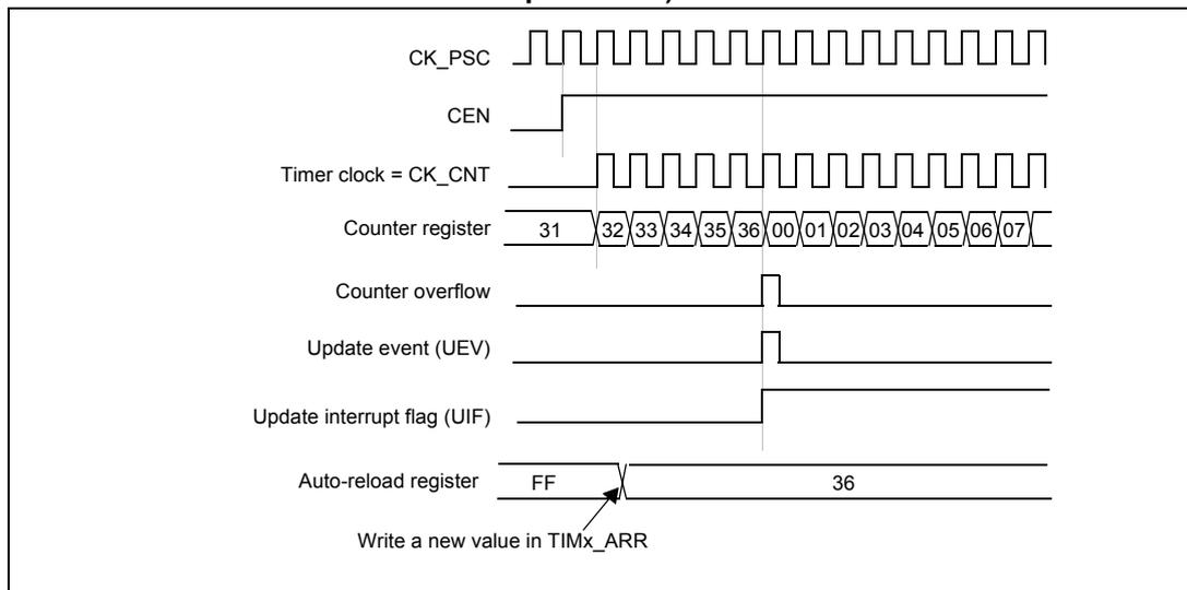
**Figure 94. Counter timing diagram, update event when ARPE=1 (TIMx\_ARR preloaded)**
