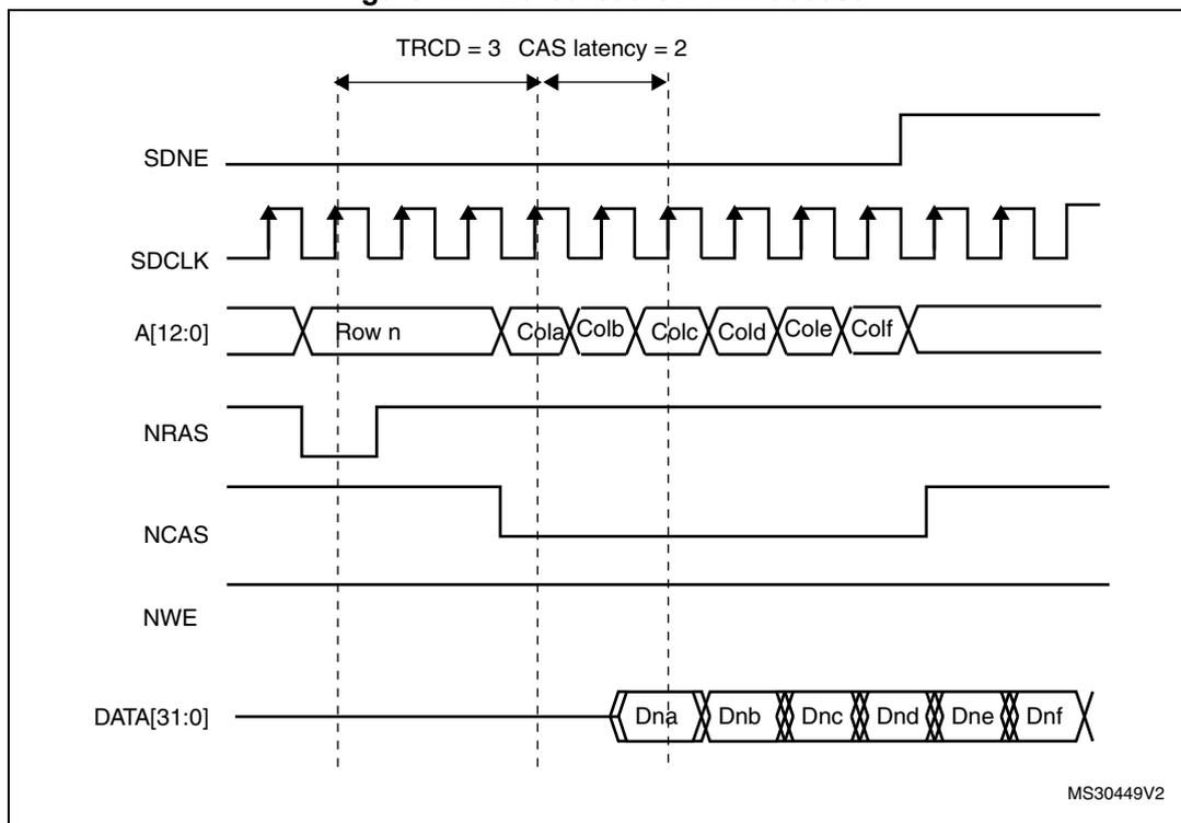
The FMC SDRAM controller features a Cacheable read FIFO (6 lines x 32 bits). It is used to store data read in advance during the CAS latency period (up to 3 memory clock cycles, programmed FMC\_SDCRx) and during the RPIPE delay (up to 2xHCLK clock cycles as configured in FMC\_SDCR1). The RBURST bit must be set in the FMC\_SDCR1 register to anticipate the next read access.
