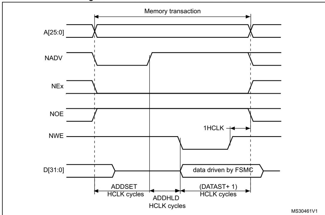
The differences with mode1 are the toggling of NOE that goes on toggling after NADV changes and the independent read and write timings.
