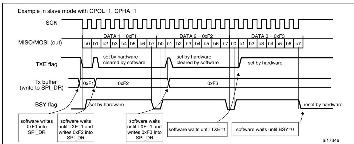
**Bidirectional transmit procedure (BIDIMODE=1 and BIDIOE=1)**
