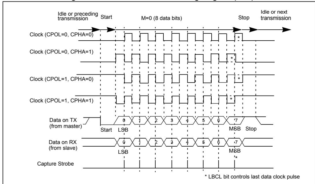
Figure 309. USART data clock timing diagram (M=1)
