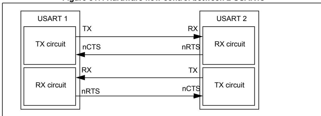
RTS and CTS flow control can be enabled independently by writing respectively RTSE and CTSE bits to 1 (in the USART\_CR3 register).
