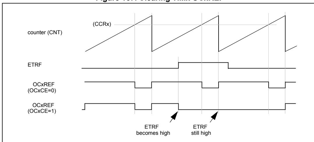
1. In case of a PWM with a 100% duty cycle (if  $CCR_x > ARR$ ), OCxREF is enabled again at the next counter overflow.
