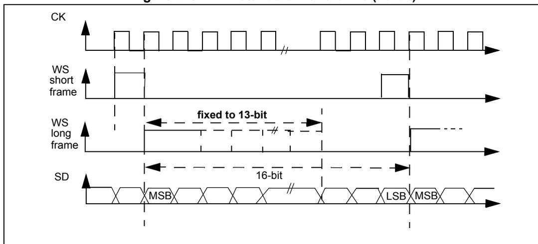
For long frame synchronization, the WS signal assertion time is fixed 13 bits in master mode.
