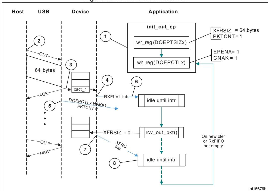
After a SetConfiguration/SetInterface command, the application initializes all OUT endpoints by setting CNAK = 1 and EPENA = 1 (in OTG\_FS\_DOEPCTLx), and setting a suitable XFRSIZ and PKTCNT in the OTG\_FS\_DOEPTSIZx register.
