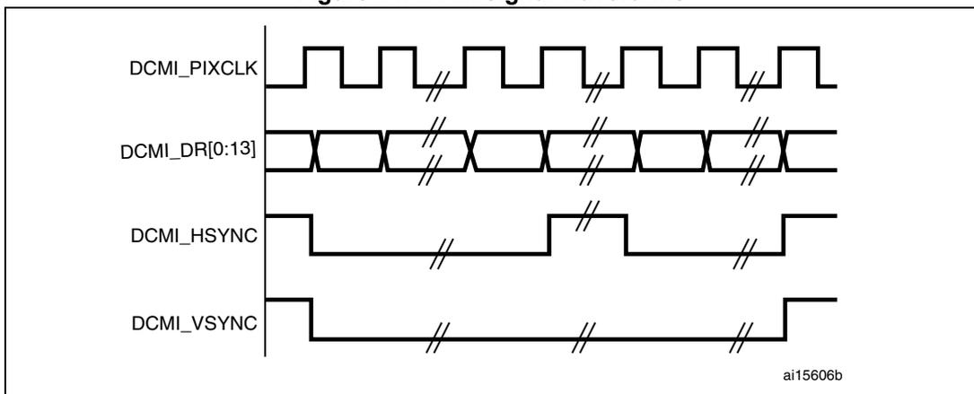
1. The capture edge of DCMI\_PIXCLK is the falling edge, the active state of DCMI\_HSYNC and DCMI\_VSYNC is 1.
