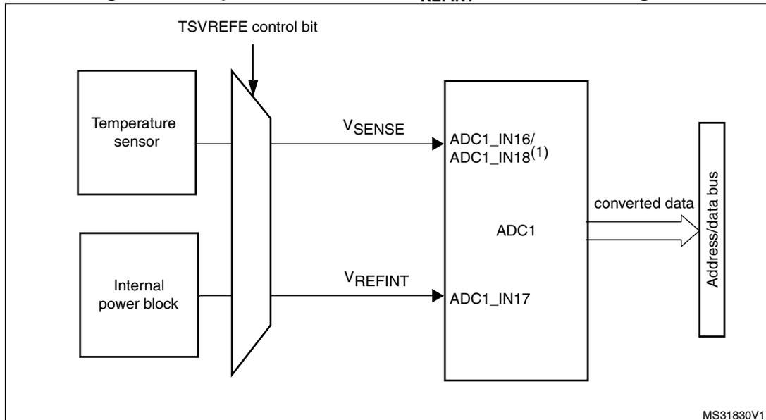
1. V<sub>SENSE</sub> is input to ADC1\_IN16 for the STM23F40x and STM32F41x devices and to ADC1\_IN18 for the STM23F42x and STM32F43x devices.
