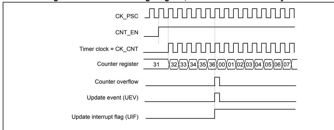
**Figure 185. Counter timing diagram, internal clock divided by 2**
