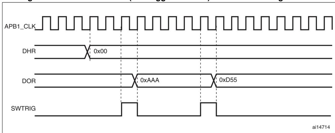
Note: The DAC trigger must be enabled for noise generation by setting the TENx bit in the DAC\_CR register.
