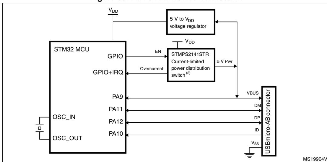
1. External voltage regulator only needed when building a V<sub>BUS</sub> powered device
