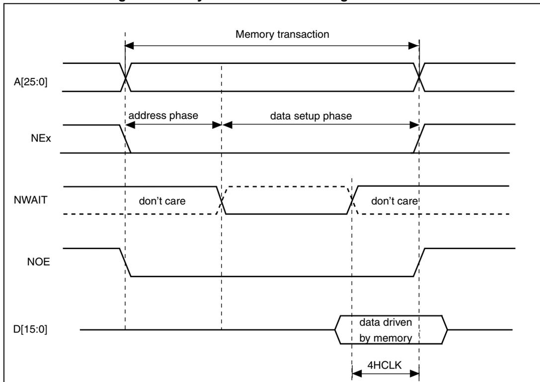
1. NWAIT polarity depends on WAITPOL bit setting in FSMC\_BCRx register.
