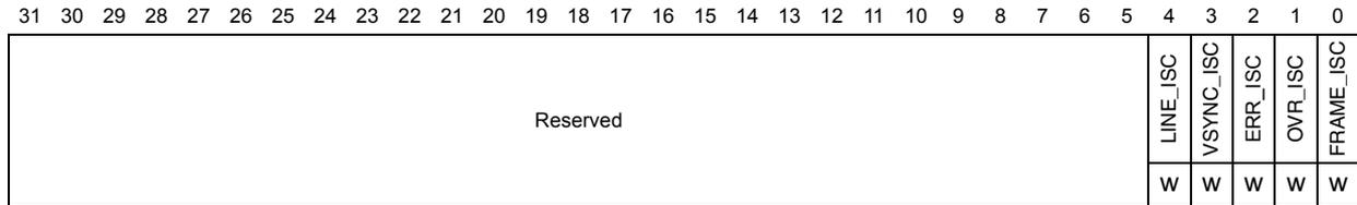
The DCMI\_ICR register is write-only. Writing a '1' into a bit of this register clears the corresponding bit in the DCMI\_RIS and DCMI\_MIS registers. Writing a '0' has no effect.
