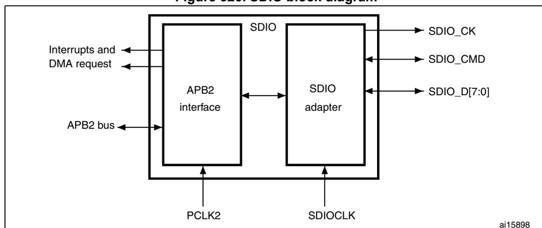
By default SDIO\_D0 is used for data transfer. After initialization, the host can change the databus width.
