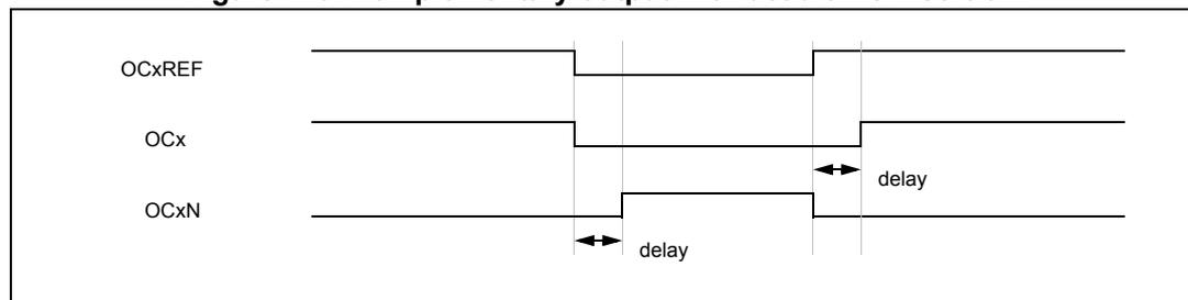
**Figure 121. Dead-time waveforms with delay greater than the negative pulse.**
