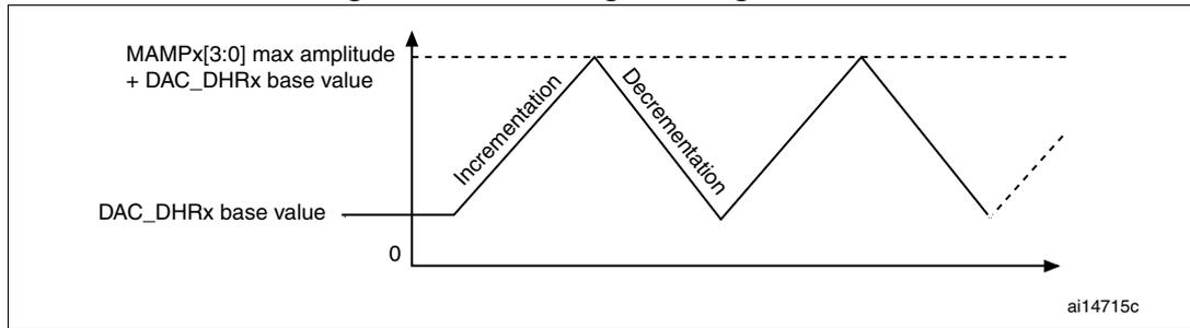
Figure 71. DAC conversion (SW trigger enabled) with triangle wave generation
