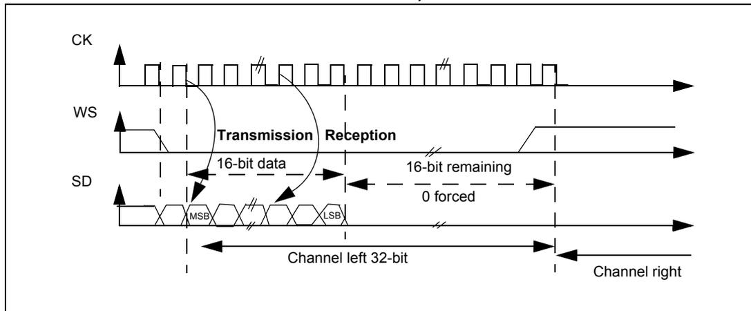
When 16-bit data frame extended to 32-bit channel frame is selected during the I<sup>2</sup>S configuration phase, only one access to SPI\_DR is required. The 16 remaining bits are forced by hardware to 0x0000 to extend the data to 32-bit format.
