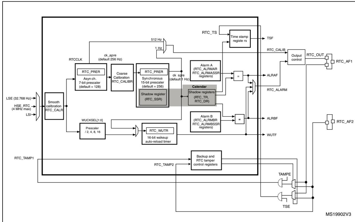
1. On STM32F4xx devices, the RTC\_AF1 and RTC\_AF2 alternate functions are connected to PC13 and PI8, respectively.
