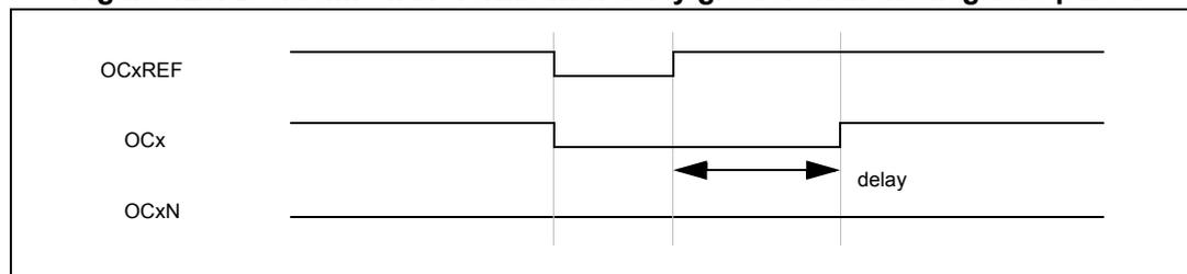
**Figure 122. Dead-time waveforms with delay greater than the positive pulse.**
