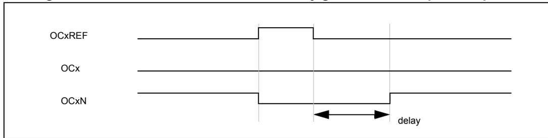
The dead-time delay is the same for each of the channels and is programmable with the DTG bits in the TIMx\_BDTR register. Refer to [Section 17.4.18: TIM1&TIM8 break and dead-time register \(TIMx\\_BDTR\) on page 572](#) for delay calculation.
