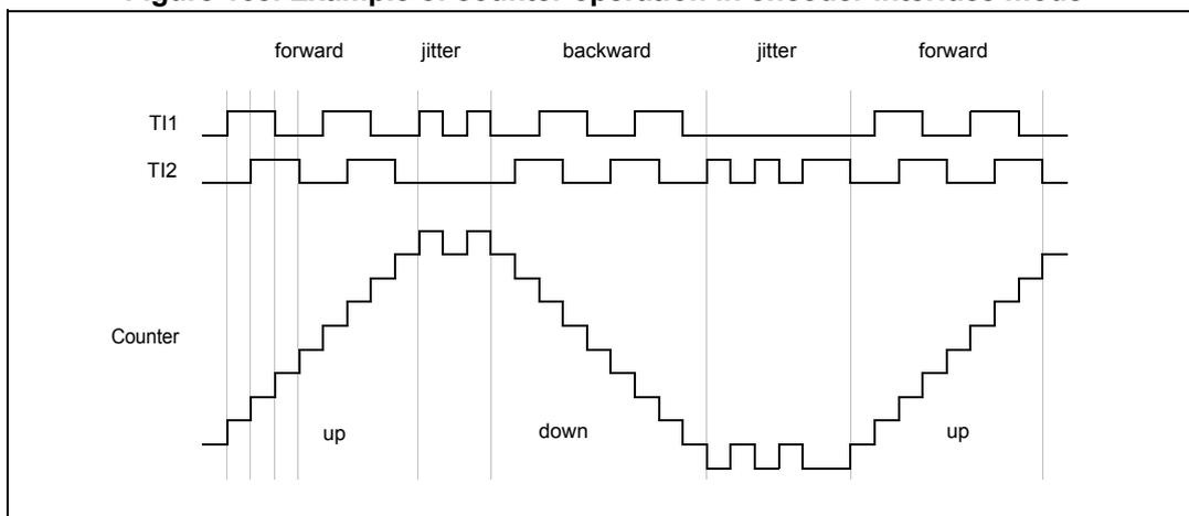
Figure 169 gives an example of counter behavior when TI1FP1 polarity is inverted (same configuration as above except CC1P=1).
