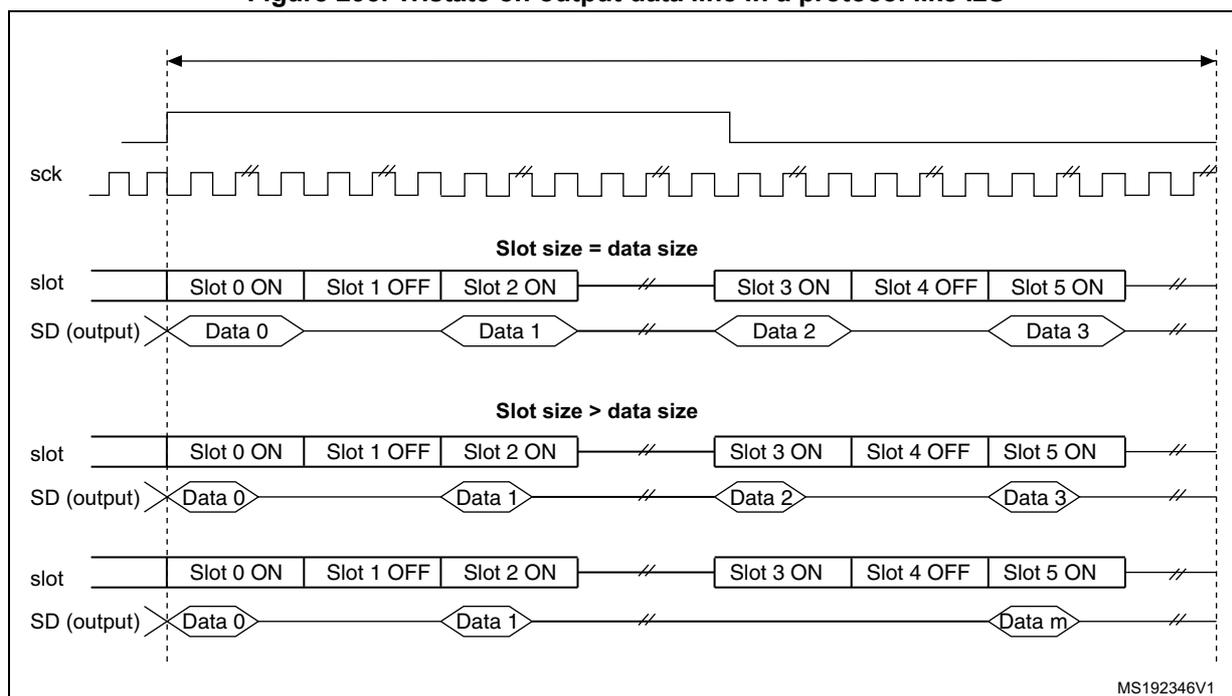
If the TRIS bit in the SAI\_xCR2 register is cleared, all the High impedance states on the SD output line on [Figure 292](#) and [Figure 293](#) are replaced by a drive with a value of 0.
