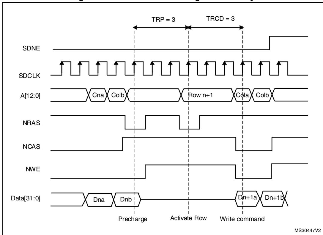
If the next access is sequential and the current access crosses a bank boundary, the SDRAM controller activates the first row in the next bank and initiates a new read/write command. Two cases are possible:
