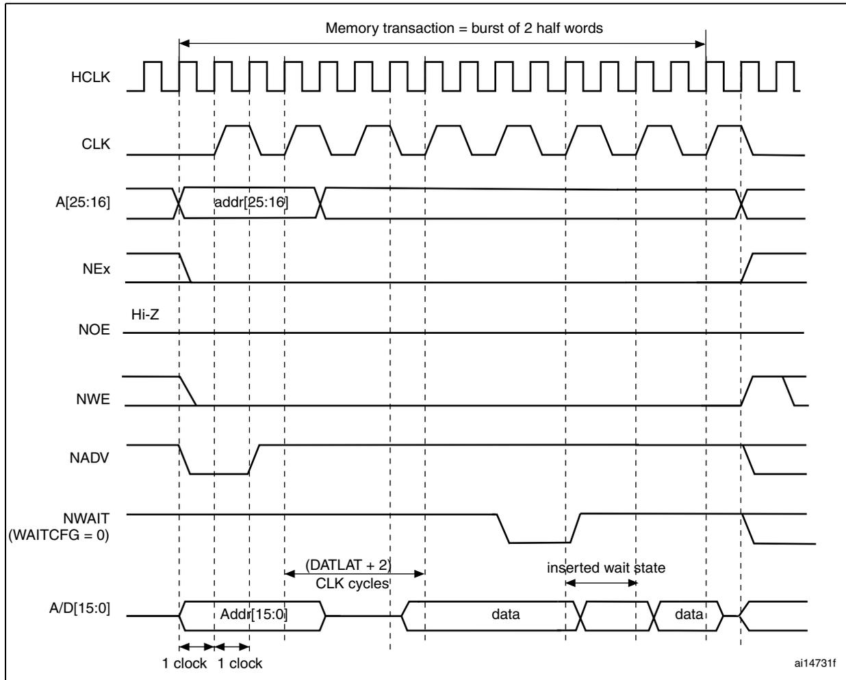
1. Memory must issue NWAIT signal one cycle in advance, accordingly WAITCFG must be programmed to 0.
