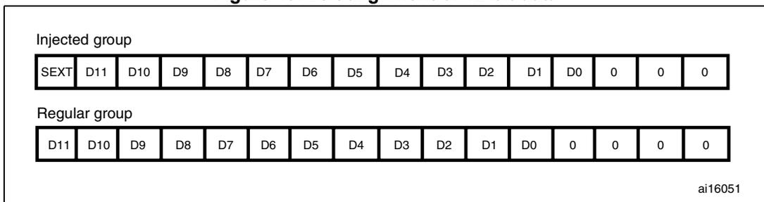
Special case: when left-aligned, the data are aligned on a half-word basis except when the resolution is set to 6-bit. In that case, the data are aligned on a byte basis as shown in [Figure 50](#).
