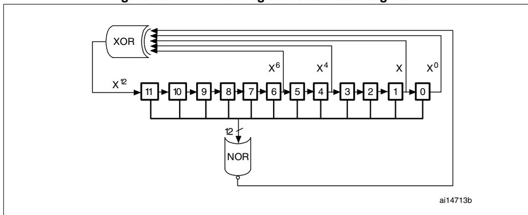
The LFSR value, that may be masked partially or totally by means of the MAMPx[3:0] bits in the DAC\_CR register, is added up to the DAC\_DHRx contents without overflow and this value is then stored into the DAC\_DORx register.
