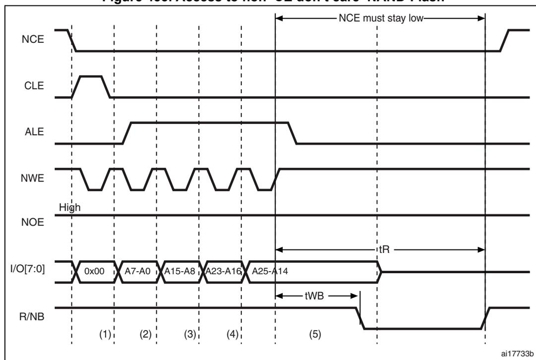
1. CPU wrote byte 0x00 at address 0x7001 0000.
