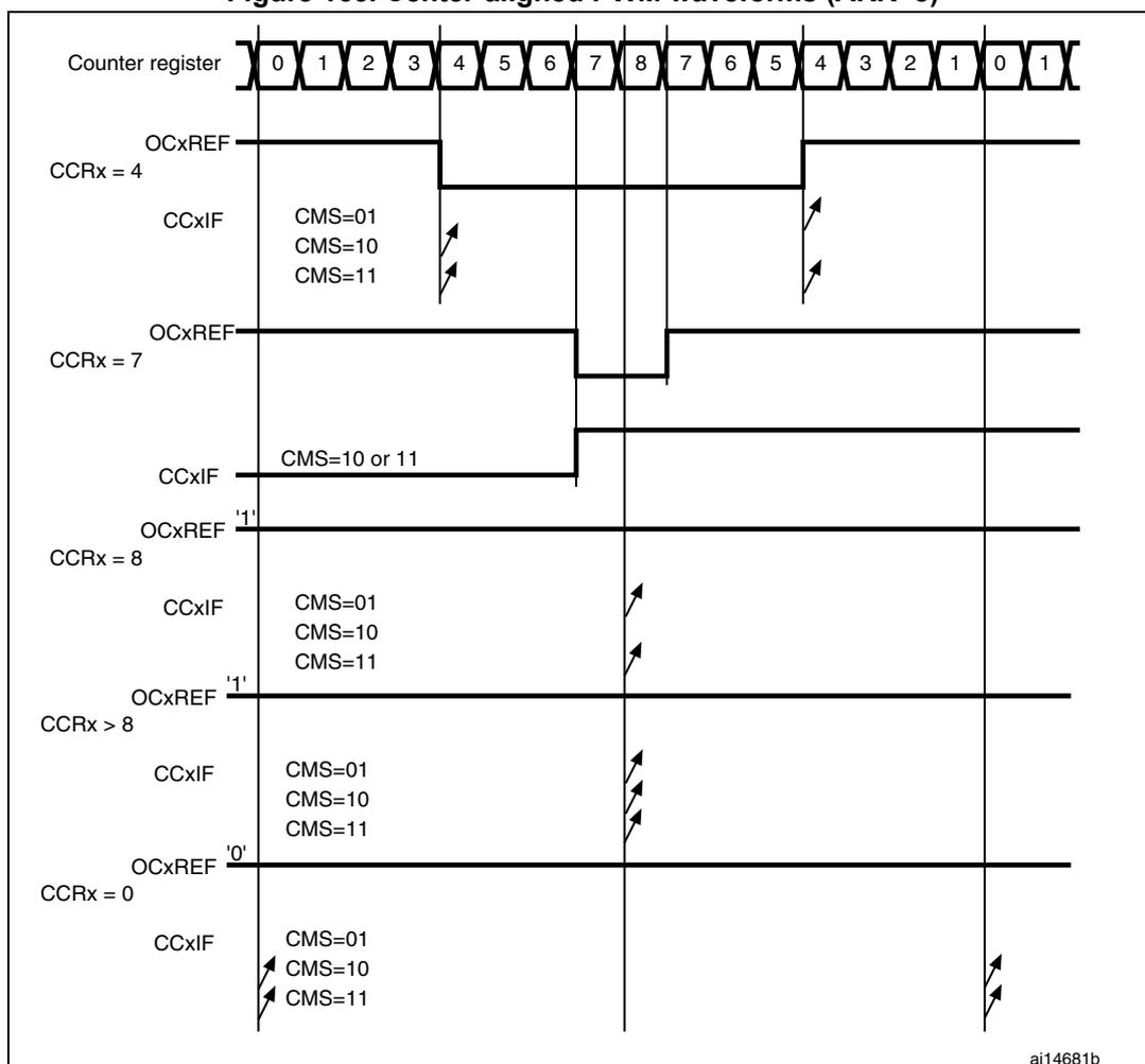
Hints on using center-aligned mode:
